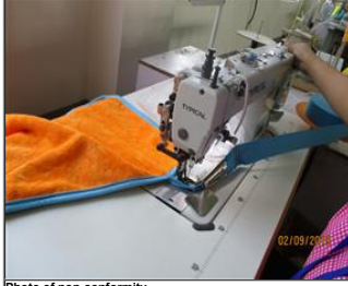
Photo of non-conformity NC-7.17 No needle protection device for the sewing machine.JPG
