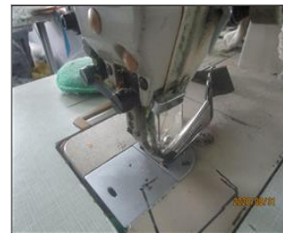
Photo of non-conformity NC 7.17 No needle protection device.JPG
